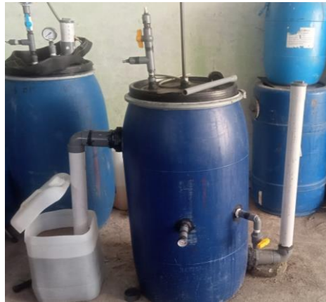
Picture 1. Manual Stirred Biodigester
